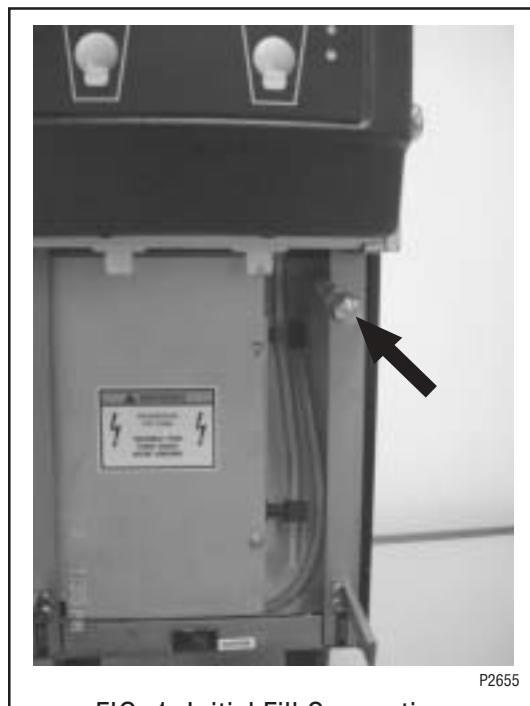
FIG 1 Initial Fill Connection
