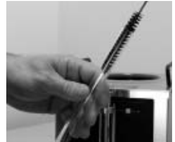
8. Clean the sight gauge with the large brush and reassemble the sight gauge.
