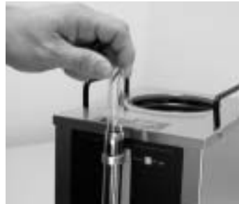
7. Remove the glass tube.
