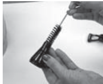
11. Use a small brush (BOM #00674.0000) to thoroughly scrub the faucet body.
