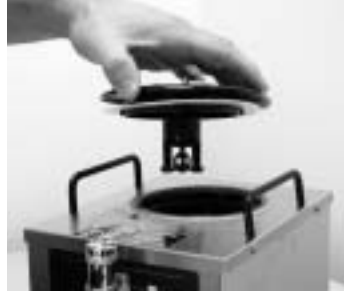
2. Pull out the lid assembly.
