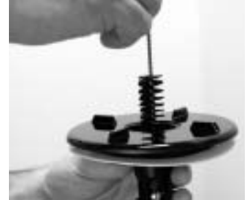
4. Clean the inlet tube with the medium sized brush and the cleaning solution.
