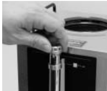
6. Unscrew the sight gauge cap.
