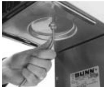
5. With the sprayhead removed, insert a deliming spring into the sprayhead tube until approximately two inches of the spring remain visible. Saw back and forth five or six times to loosen any lime deposits. Flush the tube by running a brew cycle using an empty funnel and dispenser. When the cycle is completed, replace the sprayhead.
