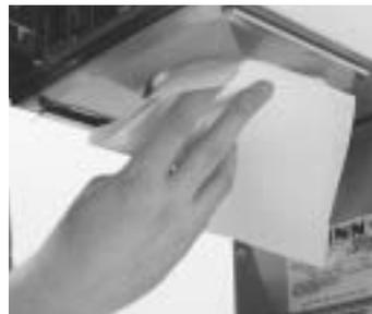
2. Use a clean damp cloth rinsed in mild, non-abrasive detergent to clean the sprayhead panel.
