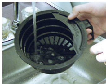
1. Clean and sanitize the funnel. NOTE: Do NOT clean this equipment with a water jet device.
