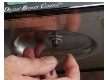
5. Use the blunt end of sprayhead cleaning tool to clean the sprayhead outlet fitting.
