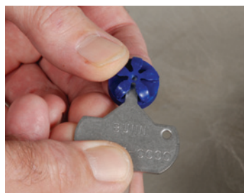
4. Use the pointed end of sprayhead cleaning tool to remove any mineral deposits from the sprayhead openings. The sprayhead openings must always remain open.
