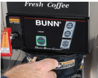
5. Slide funnel into the funnel rails of the brewer.
