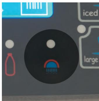
Screen will toggle between: "Empty and Clean Milk Tank, Push Rinse" and "Enter Grounds Drawer, Push Rinse". Press Rinse to complete each step.
