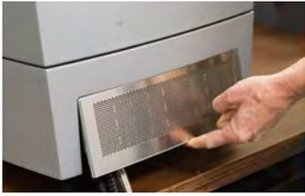
Remove the milk chiller air filter from the machine base.
