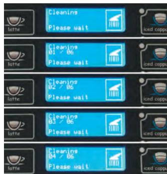
Press the Rinse key and allow the Tiger to cycle through 4 of 6 soap and soak cycles. (Allow approx. 10 min)
