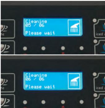
Press the rinse key - the Tiger will cycle through 2 clear water rinse cycles (6/6 total). This step is omitted with software version 3.0.2 and up.
