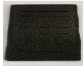
Filter must be DRY before reassembly – gently press between multiple layers of clean paper towels.
