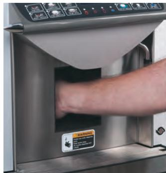
Reinsert and tighten the labyrinth (clockwise motion) and wipe out grounds drawer base area.
