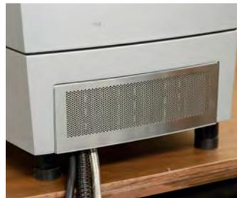
Reinstall the filter and verify that it is properly snapped in place.
