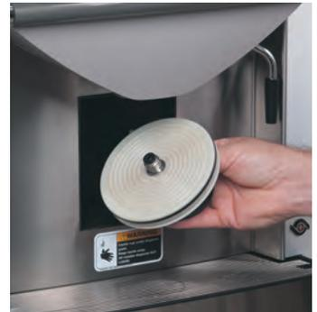
Unscrew the labyrinth from the Thermoblock. (counter-clockwise motion)
