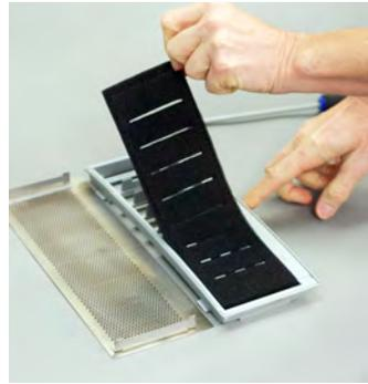
Remove filter media from the frame and rinse carefully with tepid water.
