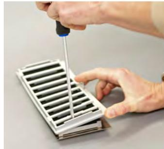
Gently bend the tabs of the outer bracket inward and press it out.
